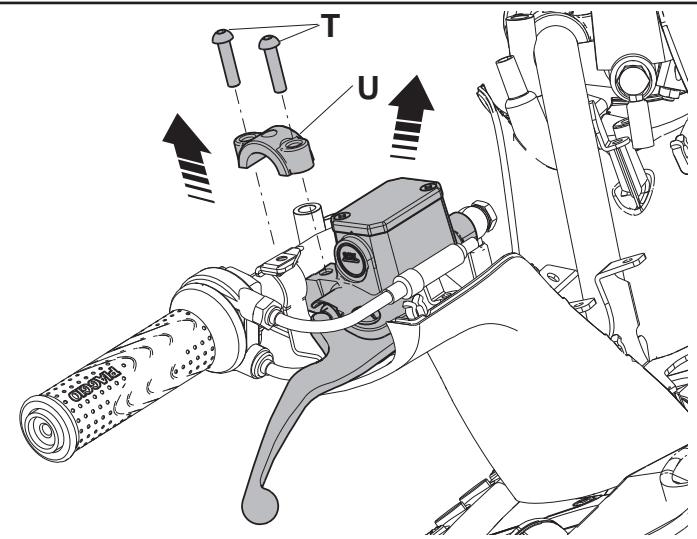
**GB** Undo the screws **T**, then remove the brake pump support **U** and detach the brake pump towards the centre of the handlebar.
