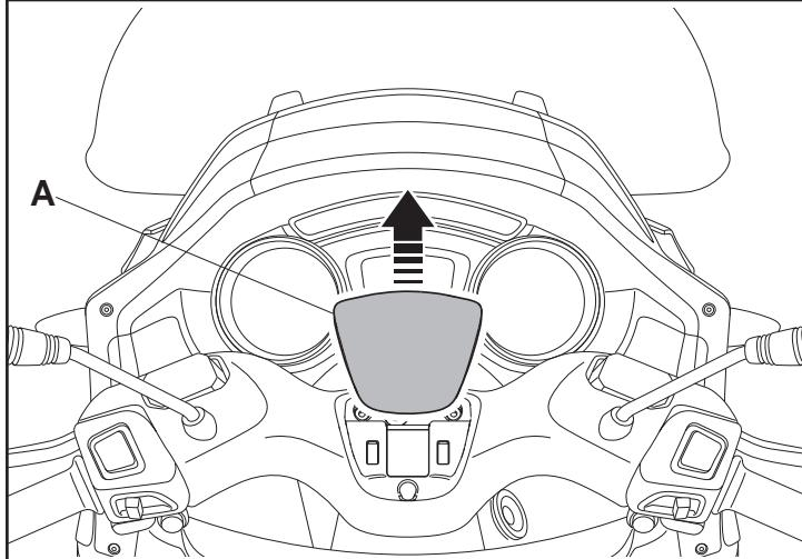
Detach the central cover **A** from the snap-fitting seat on the handlebar cover.
