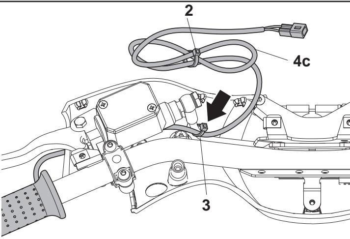
**GB** Fix the cable **4c** to the brake tube using a long clamp **3**.
