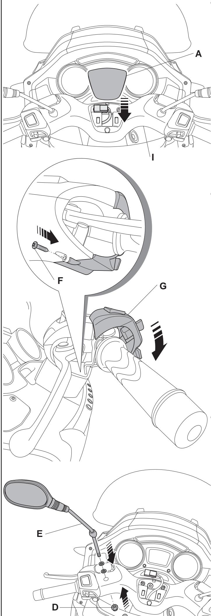
**G** Fit and fasten the cover panel **A** onto the upper handlebar cover **I**.
