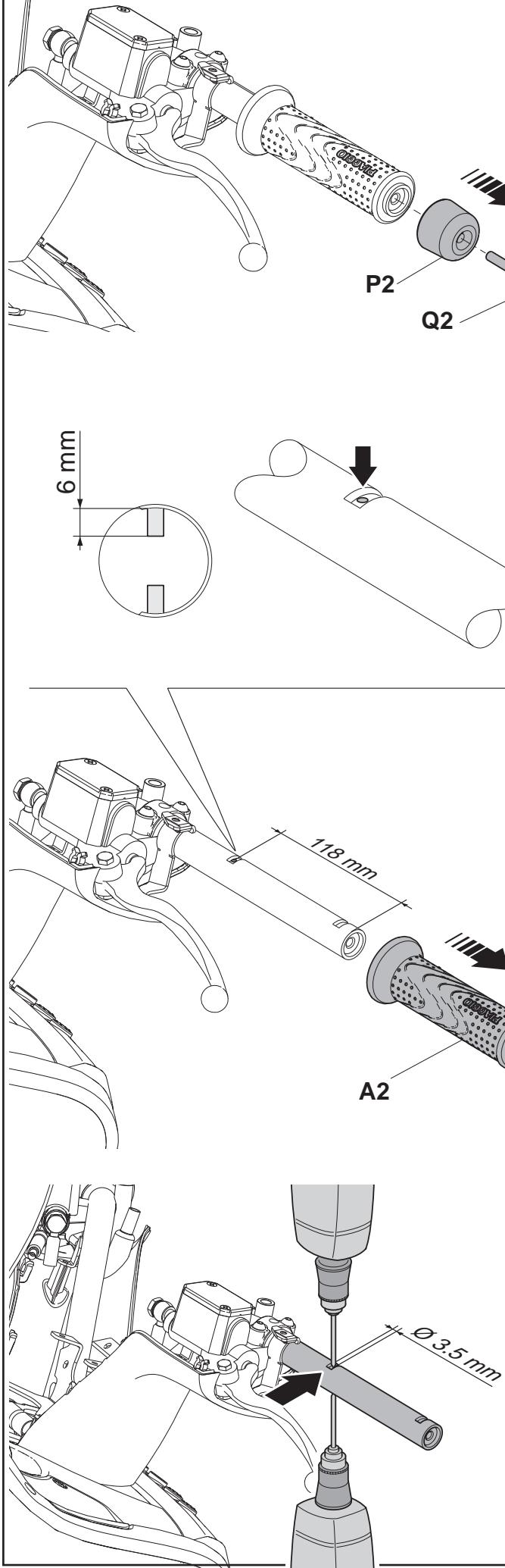
**G** To correctly drill the second hole, temporarily mount the handle grip 4, provided with the kit.
