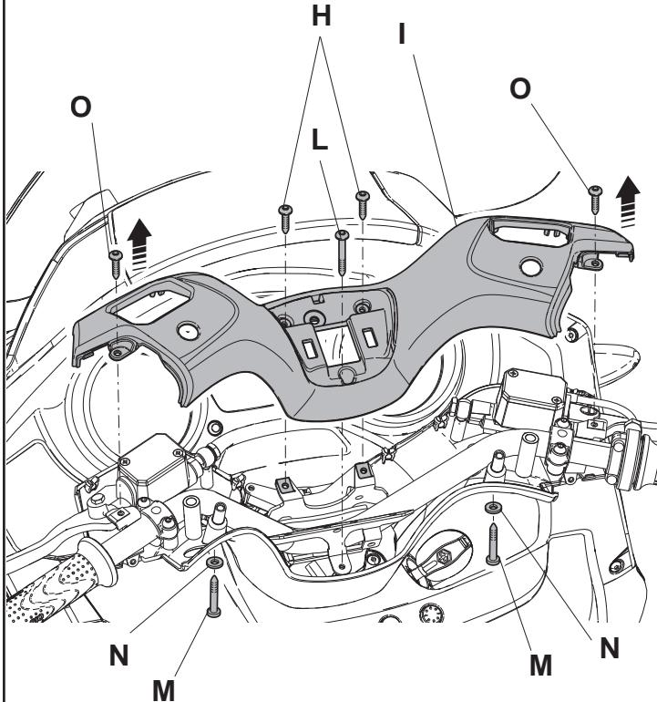
**GB** Remove the 2 screws **H** and the screw **L** located under the cover **A** removed previously, the 2 screws **M** together with washers **N** under the handlebar, and the 2 screws **O** underneath the switchgear sets removed previously.
