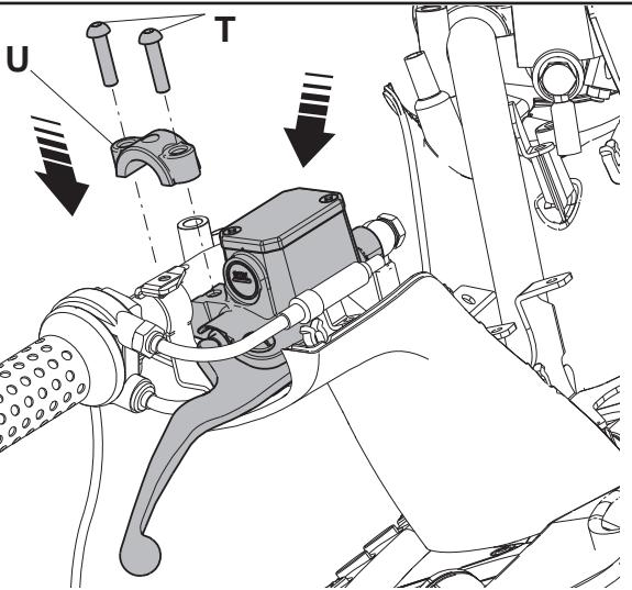
**GB** Place the brake pump again in its appropriate seat, then refit the support **U** and fix it with the screws **T**. Partially secure the screws **T**.
